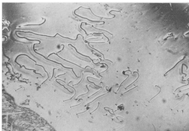
Figure 11 Free drop; formation of disclination lines more or less parallel to alignment (as inferred by contrast investigation between crossed polars); their length increases with time. Unpolarized light
